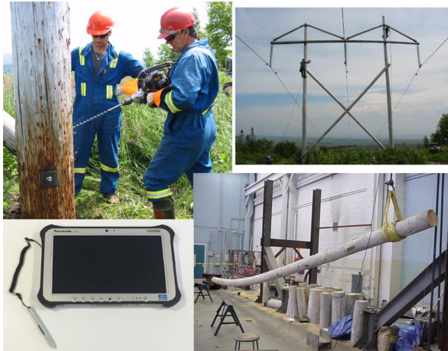
Figure 1: WPLM Inspection Techniques. Clockwise from Bottom Left: (1) Typical Field Data Collector, (2) Installing Boron Treatment, (3) Climbing Inspection, (4) Destructive Testing at MUN.
