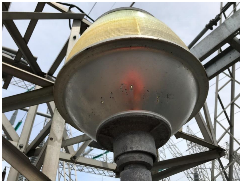
Figure 14: Light Fixture Showing Perforations due to Corrosion, Enabling Moisture Ingress
