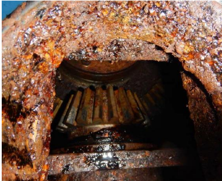
Figure 10: Transfer Case Corrosion - Burnt Dam
