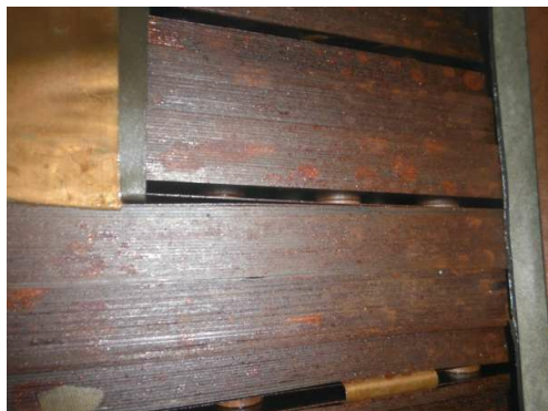
Rust formation on the top yoke near leg one.
