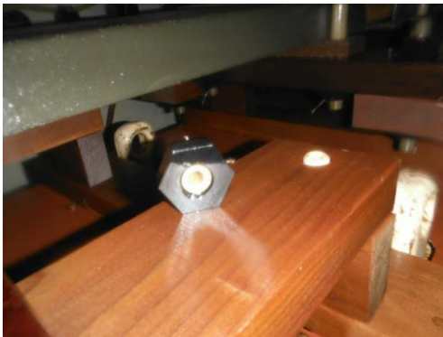
Broken stud on the top LV lead structure. The stud was not able to be repaired at the time as most of the lead work on the top of the yoke would have to be removed.
